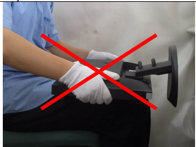
The panel is placed facedown on the lap. That may cause "Mura."
