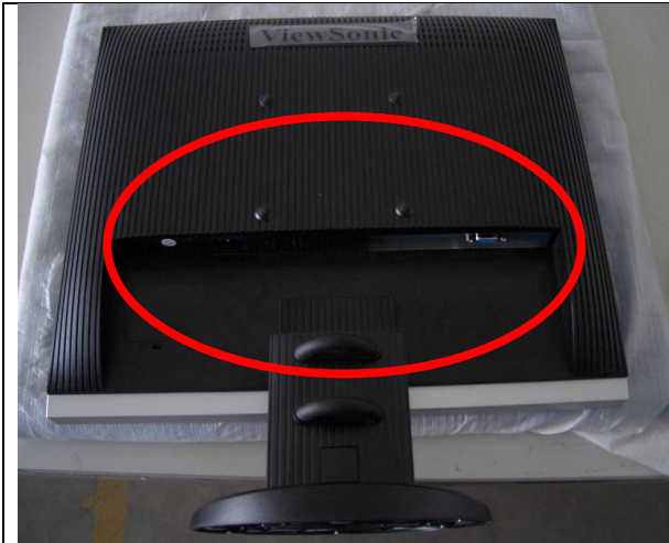
Place the monitor on the lap, the panel surface must be upwards.
